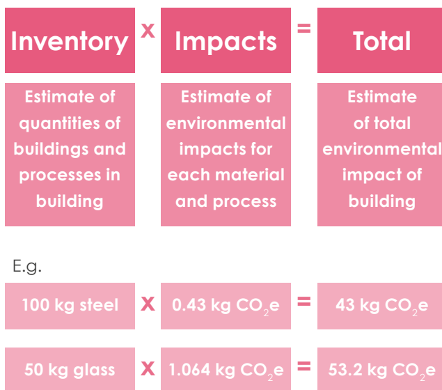
Figure A.3.1 – Simple example of LCA calculation process (Source: Carbon leadership forum practice guide 2019 p11)
